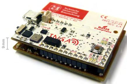
Figure 2. INGA sensor node, extended by a Bluetooth shield.
