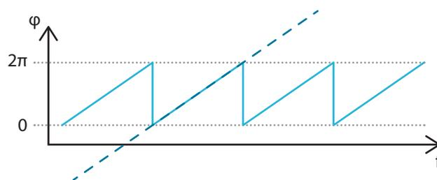
Figure 1: Ideal phase response from PMU used for distance calculation. The indicated slope is proportional to the distance between the nodes.
