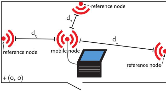
**Figure 2: Example deployment of our system. Three nodes are used as *reference nodes*. A fourth node is connected to a mobile device.**
