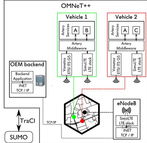
Figure 2. Architecture of the *ArteryLTE* simulation framework.
